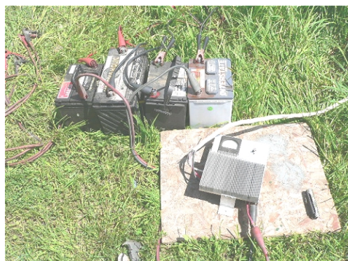
Four borrowed car batteries make up our 48 volt battery bank for testing, and a rectifier assembly with ammeter and shutdown switch change the 'wild AC' output of the wind turbine into usable form.
