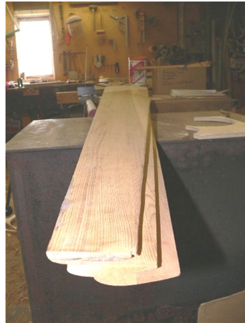
Three nicely carved blades, with a bit of epoxy and sawdust mix added to fill the voids.
