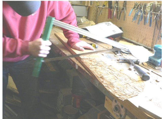
A coarse-toothed bow saw turned out to be an easy way to make the straight, deep kerfs at the blade roots.
