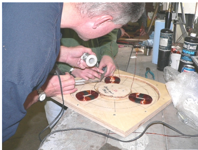
Wiring the first phase coils in series. We do it in the mold so all the wire lengths all come out right.
