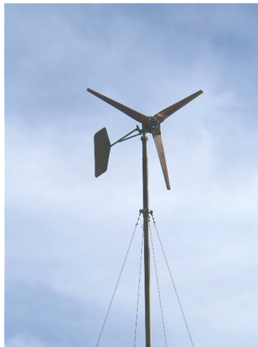
A nice little 10 foot wind turbine flying on the test tower. It spun up to 1 kW output quickly in the strong breeze we had, exceeding our expectations.
