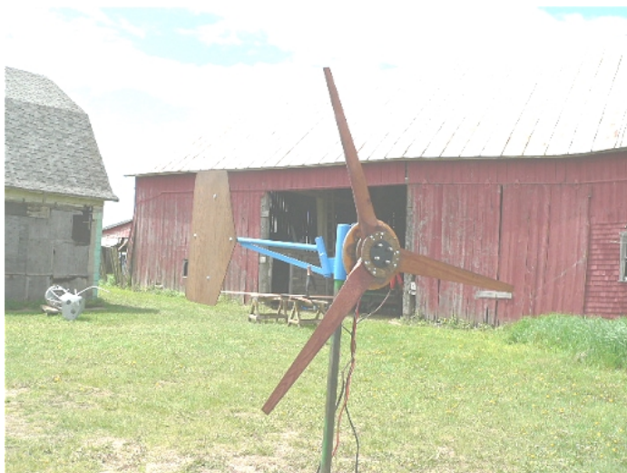
The cute little 7-foot machine, ready to begin its nationwide tour of renewable energy fairs with the MREA. Don't let turbines spin on the test stand! Short them out and tie the blades down.
