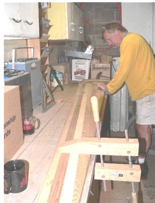
Clay from the MREA uses a mallet and chisel on a 7.5 foot blade to remove wood chunks that were kerfed out with the bow saw.
