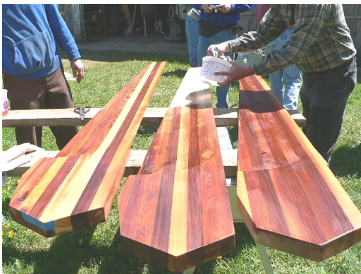
The 7.5 foot blades for the 15 foot turbine were daunting in their size and how much material had to be removed while carving – but the finished product was beautiful! Here the big blades are getting their first coat of finish.
