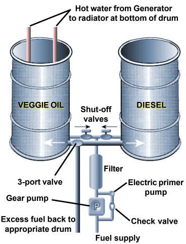
A rear heater core of of a schoolbus was first set in the bottom of the 55 gallon drum connected to the heater hoses and attaching the fuel pickup line to it.
