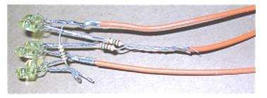
After the soldering is done the large disk with the magnet ring is replaced and a quick spin of the shaft should light the LEDs!
