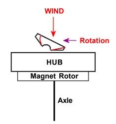
Some rulers have a lower or higher angle than others. This set of blades has 2 layers of a business card under one side of each blade to increase the angle as viewed from the end. About 8 degrees seems like a good angle. After the blade angles are adjusted if they needed it, a bit of wood glue is a good idea.
