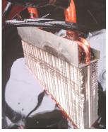
Water fittings were then welded to the sides. Engine coolant was run through this homemade water jacket.
