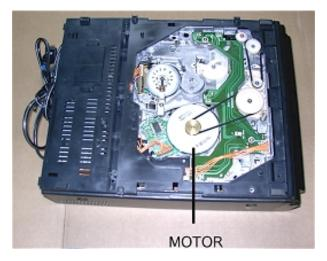
The large disk on the front of the motor was held in place by magnets and a small plastic washer on the axle. Often the shaft can be pushed, removing the assembly as the washer slides down the shaft, but sometimes they need to be cut off. Save the washer if it comes off easily.
