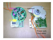
Each phase has the same Ohm reading. This 'good' one is about 4 ohms, so from the common to any output is 4 Ohms. From any output to any other output will be 8 Ohms.
