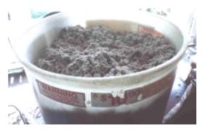
There are floors in some very old house attics. Cellulose works very well for insulating under these. There is usually some open area around the perimeter where you can run the hose under the flooring, then pull the hose back as the space fills with insulation. When you are filling these hidden spaces, it is a smart practice to count how long they take to fill up. Then, if one takes longer, shut the machine off!
