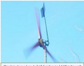
This photo shows a home-built 17-foot diameter 3.5 kW turbine with the tail in fully furled position. The machine is still making near maximum power, but it facing at an angle into the wind to reduce wind input. Photo by Dan Bartmann.
