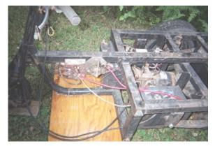
If you you don't have facilities or the ability to weld, then you can save a lot of money by just cutting the steel to length and getting it ready for a welder to do the job for you without wasting time. Just check that everything fits together well with the transaxle, front end, battery shapes, etc. before taking it all to be welded. It cost me just \$27 for the steel, and I bartered with a friend for the welding, so the new chassis was almost free!
