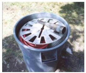
The blower will probably come with its hose and cord in a trash can. The can is handy to use as a receptacle for breaking up the insulation by hand before dumping into the blower. This is a recommended step to avoid clogs when insulating walls. There is usually also a blower switch on a long cord, this being for the person who handles the hose.
